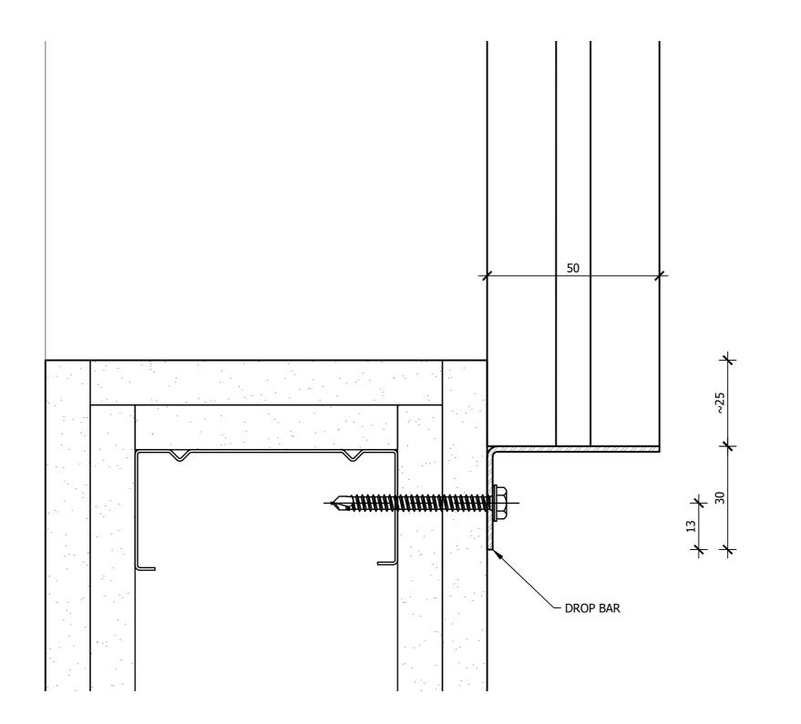
**WINDOW SILL BOTTOM BAR DETAIL** SCALE: 1:1 @ A2
